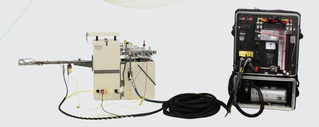
The Apex Instruments Method 23 (Modified Method 5) source sampling kit is utilized for Method 23 Determination of Dioxins and Furans (D/F's) and/or Method 0010 Determination of Semi-Volatile Organic Compounds. The sampling train is identical to the standard Method 5 system with the addition of a water-cooled glass condenser and an XAD absorbent module followed by a knockout impinger.
