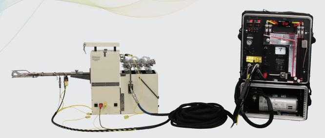
The Apex Instruments Method 26A sampling train is used for the determination of hydrogen halide and halogen emissions. Method 26A is the isokinetic alternative to Method 26. This method is particularly suited for sampling sources controlled by wet scrubbers emitting acid droplets. The method requires a Method 5 sampling train with the use of additional impingers, reagents, and PTFE-coated glass fiber filter media.
