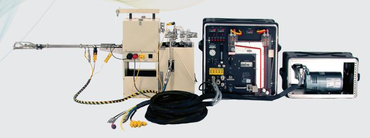
Using the Method 5 Sampling System, particulate matter is withdrawn isokinetically from the source and collected on a glass fiber filter maintained at a temperature of 120 ±14 °C (248 ±25 °F) or such other temperature as specified by an applicable subpart of the standards or approved by the administrator for a particular application. The PM mass, which includes any material that condenses at or above the filtration temperature, is determined gravimetrically after the removal of uncombined water.
